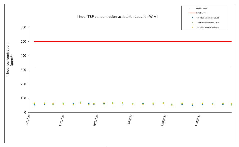
Figure 1: Graphical Illustration of Measured 1-hour TSP (μg/m³) Levels at W-A1
