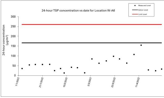
Figure 4: Graphical Illustration of Measured 24-hour TSP (μg/m³) Levels at W-A6
