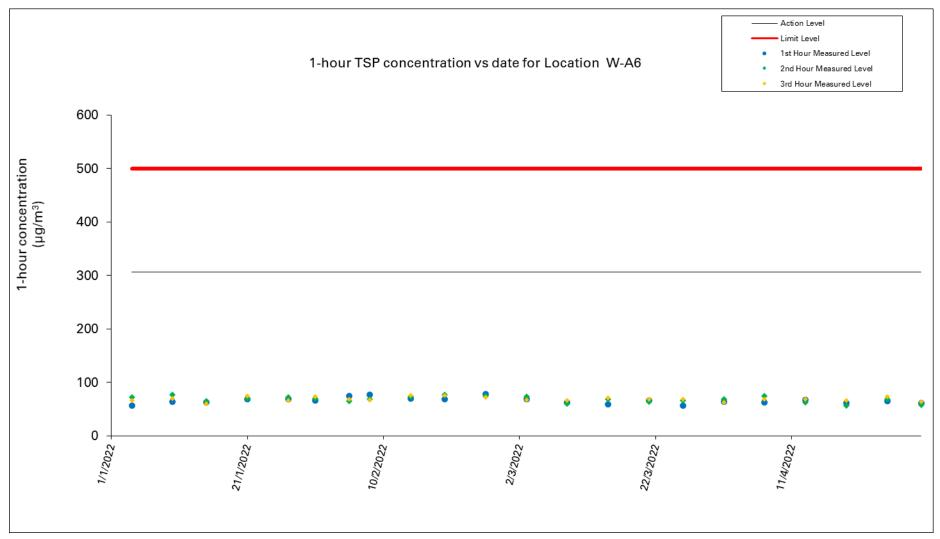
Figure 2: Graphical Illustration of Measured 1-hour TSP ( $\mu g/m^3$ ) Levels at W-A6
